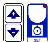
These settings refer to the operation mode of the system and must be made on initial startup. Press - / + at the same time for at least one second: the message **C.O.S.t.** will be displayed. Press then repeatedly **SET** until the message regarding the chosen variable is displayed (see table below): variable's value and message will be displayed.
