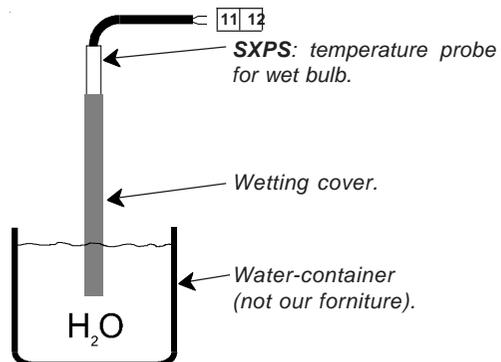
**Check periodically the sock installed on the sensor has not been clogged by calcium carbonate scale. If so, remove it then clean or replace it.**
