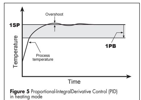
Figure 5 Proportional-Integral-Derivative Control (PID) in heating mode
