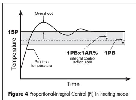
Figure 4 Proportional-Integral Control (PI) in heating mode
