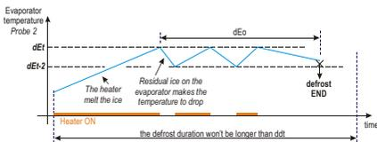
Note: if PF2 error, the defrost will be performed every dPt hours for ddt minutes, without control of dEt and dEo.
