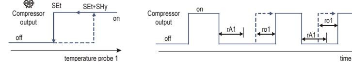
**WARNING:** during the installation, take care to set proper rA1 value to avoid compressor or relay faults.
