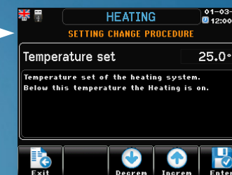
Heating temperature setting
