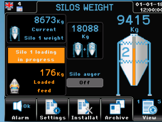
Viewing silo load
