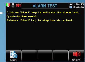
Manual alarm test
