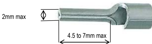
2-17 Lead Terminal for C22
